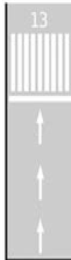
Permanently displaced (pre threshold area fit for aircraft movement)
