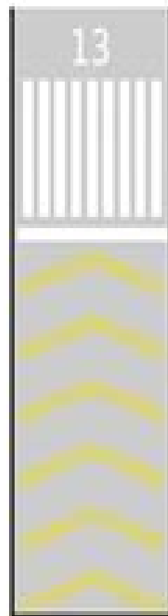
Pre threshold area fit for use by aircraft as a stopway only
