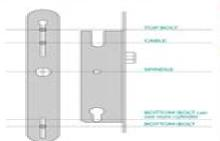
The temperal is secured by tree bolts that the through the door. The bottom bolt can use the existing hold below the suns cylinder. The top both 6 cable might require new holes.
