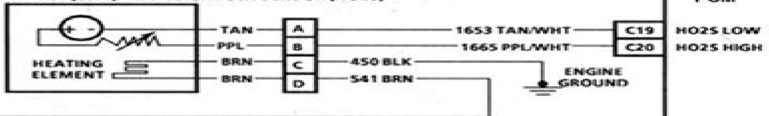
BANK 2 (RIGHT) HEATED OXYGEN SENSOR (HO2S)
