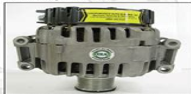
Figure 3 – This side view shows that the pad-mount bolt locations are not in a square pattern, making test bench mounting a challenge.
