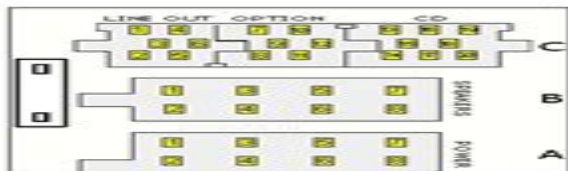
36 (20+8+8) pin Head Unit / Car Stereo ISO connector
