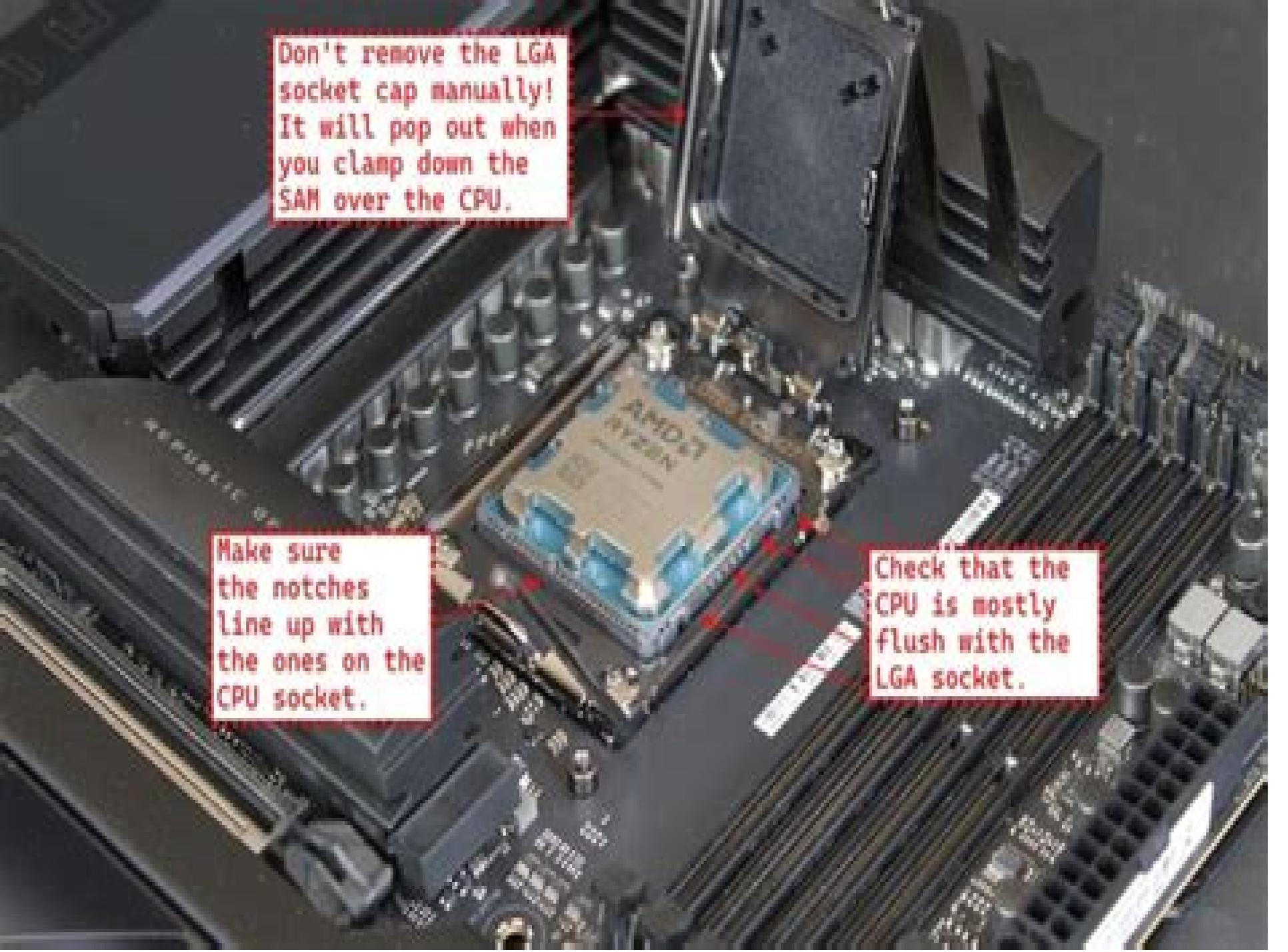
Don't remove the LGA socket cap manually! It will pop out when you clamp down the SAM over the CPU.
