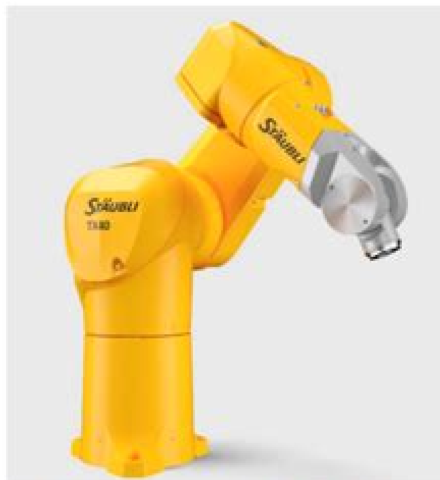
Figure 3: (a) The Staubli TX-40 robotic arm; (b) Joint axes and dimensions. All dimensions are in millimeters. Joints are numbered consecutively from 1 to 6. Frame {0} is the space frame. Frame {7} is the end-effector frame. Note: the schematic does not show joint frames – only the joint axes ( z_1, z_2, \dots, z_6 ). Recall that joint frames are not needed to calculate the kinematics with the Product of Exponentials Formula.
