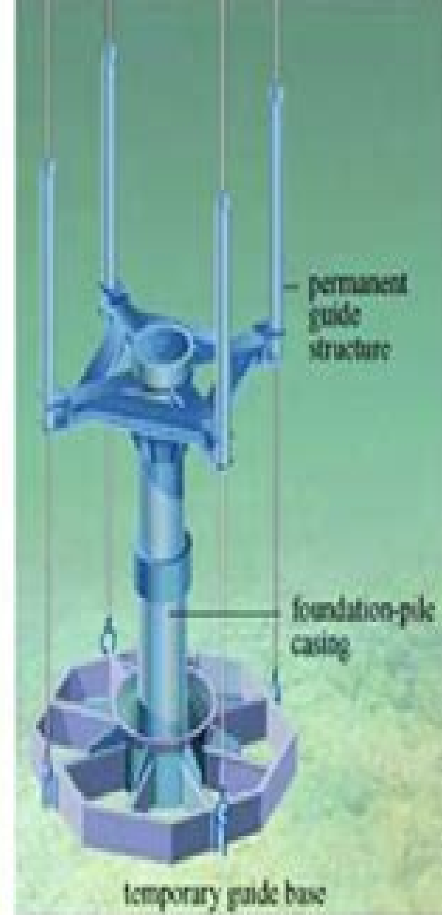
Foundation-pile casing and permanent guide structure
