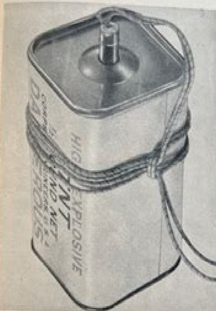
Figure 412a. Half-pound TNT block primed electrically.
