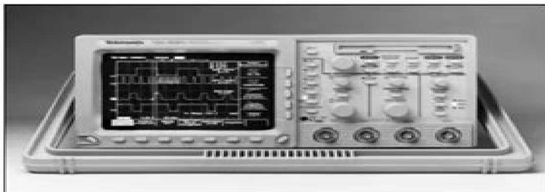
The TDS 460A 400 MHz, four channel, Personal Lab Scope.
