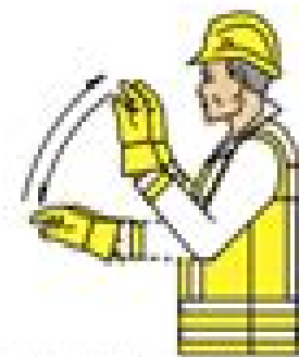
move away from bankman
