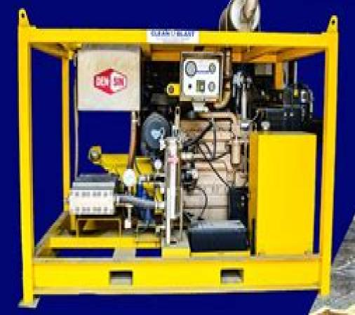
ULTRA HIGH PRESSURE (UHP) DEMO 2500 BAR DIESEL POWERED
