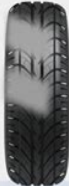
DEFECTIVE SUSPENSION OR BAD BALANCING
