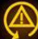
TRACTION CONTROL MALFUNCTION
