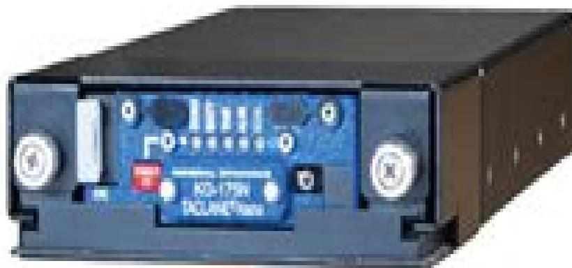
TACLANE-Nano (KG-175N) Adapter Module (for KG-175D)
