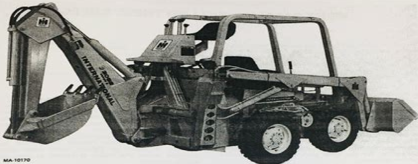
International 3082 Series B Backhoe mounted on a International 3200 Series B Tractor.
