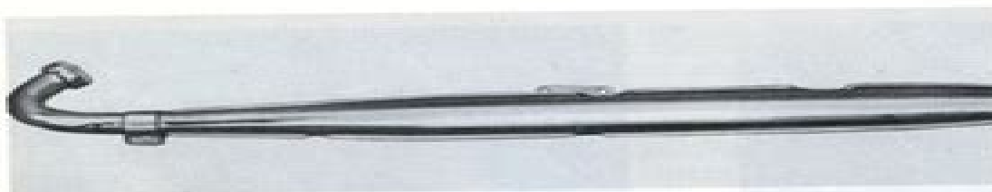
Fig. 8-1-6 Removing muffler with exhaust pipe fitted
