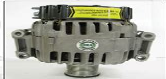
Figure 3 – This side view shows that the pad-mount bolt locations are not in a square pattern, making test bench mounting a challenge.
