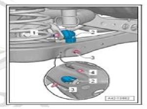
Counterhold on the internal engagement of the coupling rod when tightening the nut -1-.
