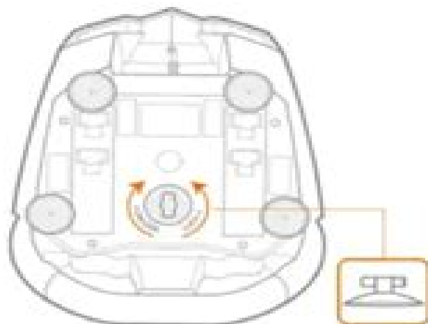
Step 1 Put the suction cups into bottom slots, then rotate to lock up the suction cups.
