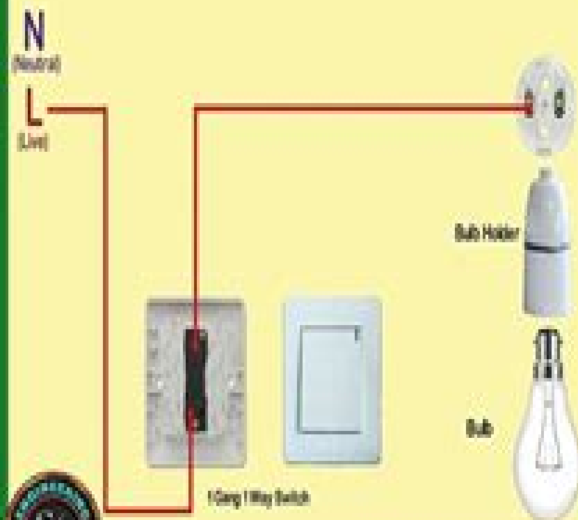
[01] 1 Gang 1 Way Switch Connection
